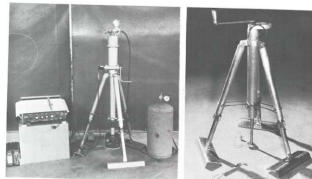
Fig. 1-7 Portable bevameter, U.S. Army Land Locomotion Laboratory. Left photo shows the shear head, right depicts the penetration plate rig. Loading device is operated by means of compressed air; xy recorder (left) plots the stress-strain curves.
